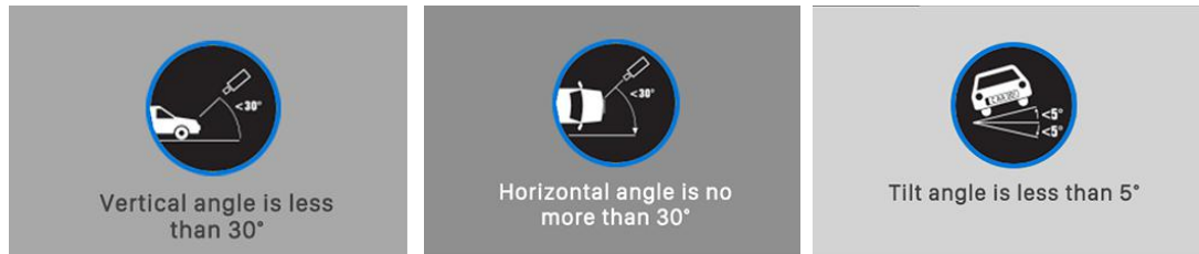
Figure 3 Installation Angle
